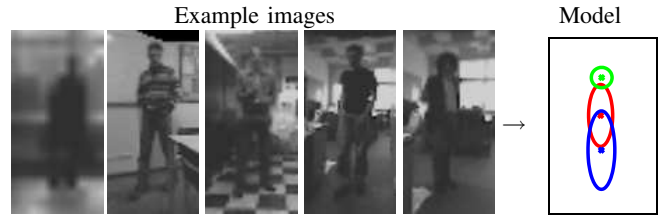
Fig. 4. Example images from the data set used to train our probabilistic part-based model and examples of learned part arrangement model parameters. For each part we present its mean position contained in the parameter \mu . The ellipse represents the 1-sigma uncertainty of the part position as described by the diagonal elements of the covariance matrix \Sigma . Here green color represents head, blue are legs and red is the full body detector.
