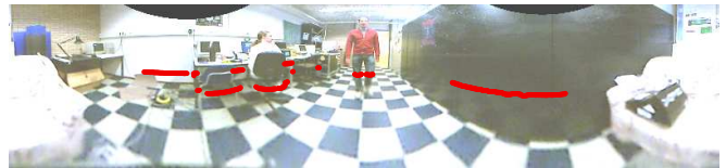
b) Corresponding panoramic image from the robot omnidirectional camera. The 2D laser range scan points from above are projected onto the image.
